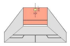
Stripes or patterns of any type will not be permitted on the wall playing surfaces except on the front wall at a min. height of 3600mm above the where a logo, club or sponsors name may be used providing it is not n 750mm square and is located central on the front wall.
