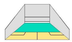
The floor shall have no more than two colours and each colour shall be bounded on at least two sides by the floor markings. The use of colours shall be symmetrical about the half court line.
