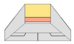
3. The front wall may be two colours, one below and one above the service line. The front wall colours need not be the same colour as the side wall colours.
